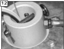
Take out pin and keeper clip and then loosen the 2 set screws on the yoke to let the downrod slip into yoke.
